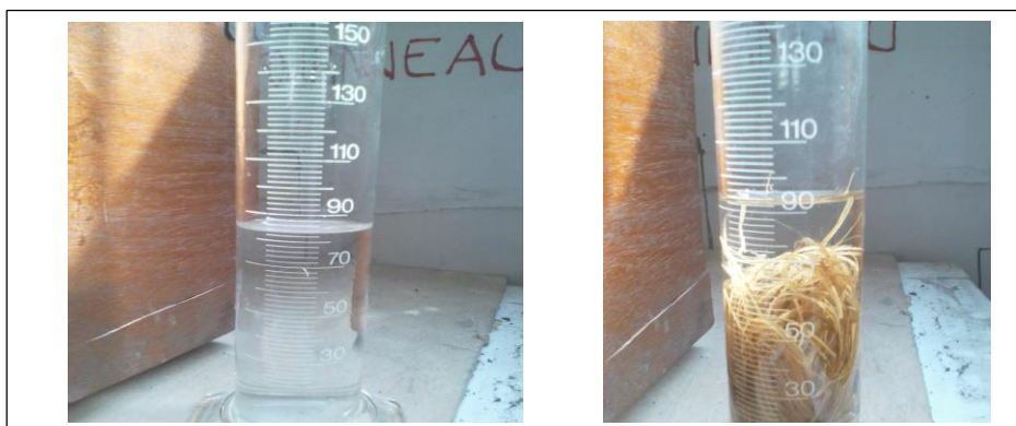
Figure 15: 15-a) Content volume: content alone; 15-b) Volume of Benzene: Benzene-Fibers.
